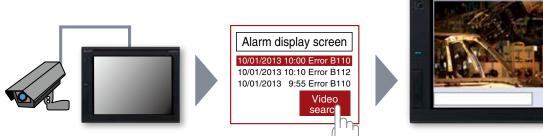
Attach a video camera to the GOT, and record the production line before and after trouble occurs.
