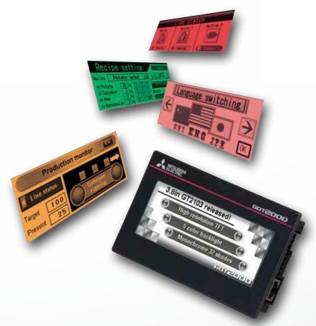
Display...... Monochrome (black/white), 32 shade grayscale TFT LCD display, 3.8"
